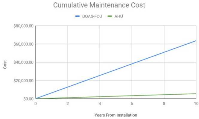
Figure 11: Yearly Progressive Maintenance Cost of Original System versus Air Handling Unit System
